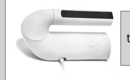
the intelligent fall sensor fearless is the basis for behavior analysis in the bathroom
