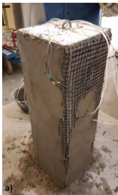
Figure 16 Retrofit of RC column. [69] Figure 17 Shear retrofit of an RC beam [85]
